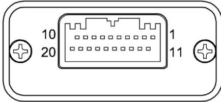
Figure 4: Amplifier Pinout
