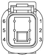
Figure 3: DTM Pinout
